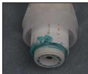
Figure 1. Salt residue build up.
