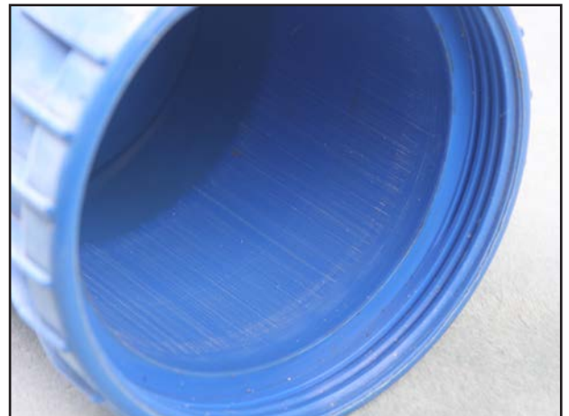
Figure 3. Scratches on the inside of the canister of an injector due to wear.
